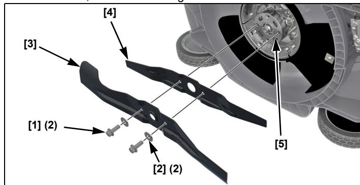
3. Use a 14 mm (6 point) socket wrench and remove the two cutting means bolts [1] and special washers [2] from the cutting means control assembly [5]. Use a wooden block to prevent the cutting means from turning when removing the bolts.
