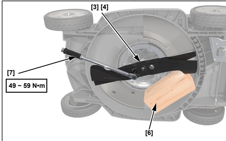
**Cutting means bolt torque: 49 ~ 59 N·m**
