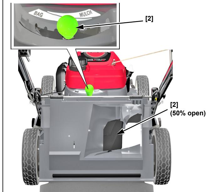
Maximum rear discharge will occur when the Clip Director knob is all the way to the left (BAG) position. As the Clip Director knob is moved toward the right (MULCH) position, less grass will be discharged through the rear discharge guard.
