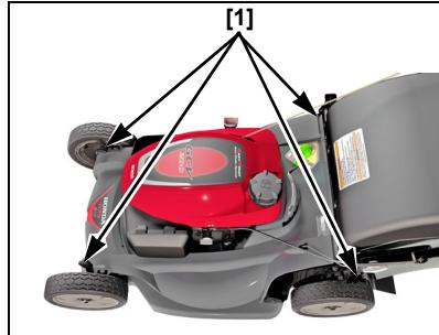
To adjust cutting height, pull each adjustment lever [1] toward the wheel, and move it into another notch.
