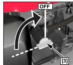
3. When the mower is not in use, turn the fuel valve [3] to the OFF position.
