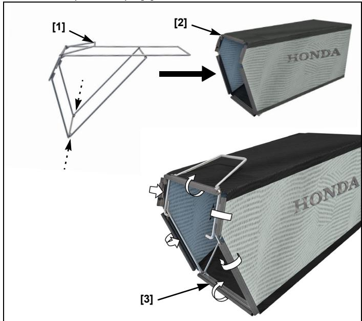
2. Lift the discharge guard [4] and install the grass catcher [2].
