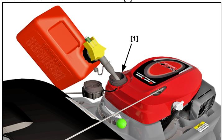
After refueling, tighten the fuel tank cap securely.
