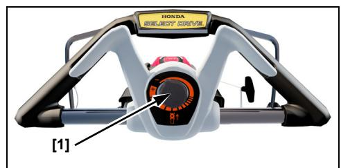
You can reduce the ground speed by partially releasing the Select Drive control.
