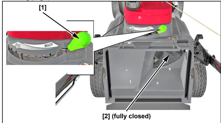
If a high resistance is noticed when moving the Clip Director knob from side-to-side, excessive grass may have built up on top of the sliding door.
