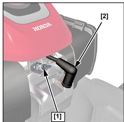
3. Inspect the spark plug. Replace it if the electrodes are worn or if the insulator is cracked or chipped. Clean the spark plug with a wire brush if you are going to reuse it.
