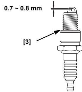
4. Measure the spark plug electrode gap with a suitable gauge. The gap should be 0.7 ~ 0.8 mm. Correct the gap, if necessary, by carefully bending the side electrode.
