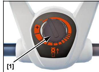
**MAX** will propel the lawnmower at its fastest speed.
