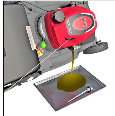
Please dispose of used motor oil and the containers in a manner that is compatible with the environment. We suggest you take it in a sealed container to your local recycling center or service station for reclamation. Do not throw it in the trash, pour it on the ground or pour it down a drain.
