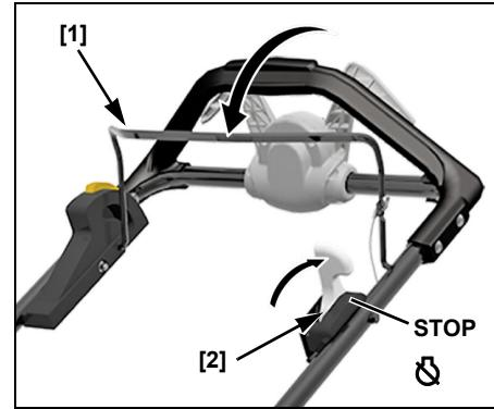
2. Move the throttle lever [2] to the STOP (⤠) position to stop the engine.
