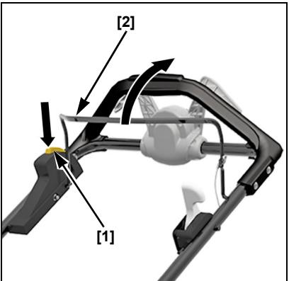
Continue to hold the cutting-means control lever against the handlebar to maintain cutting means rotation. Always keep the cutting-means control lever fully engaged while mowing. Do not partially disengage - doing so will reduce the life of the clutch system.
